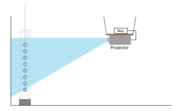
Tube should be placed in corner with projection aimed at it. Mini Mac should feed video into projector.
