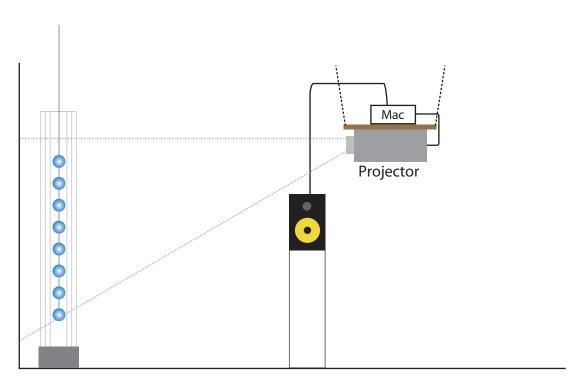
Speakers should be on pedestals, at ear level. Use cabling to feed audio from computer to speakers.
