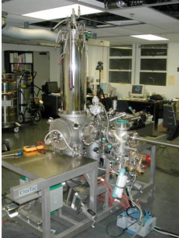
Figure 3. View of a Scanning Tunneling Microscope (STM) at the PICO lab of one of the authors (Gimzewski) at UCLA.
